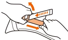
When the belt is hard to pull, lift up the buckle and pull down as shown in diagram.
